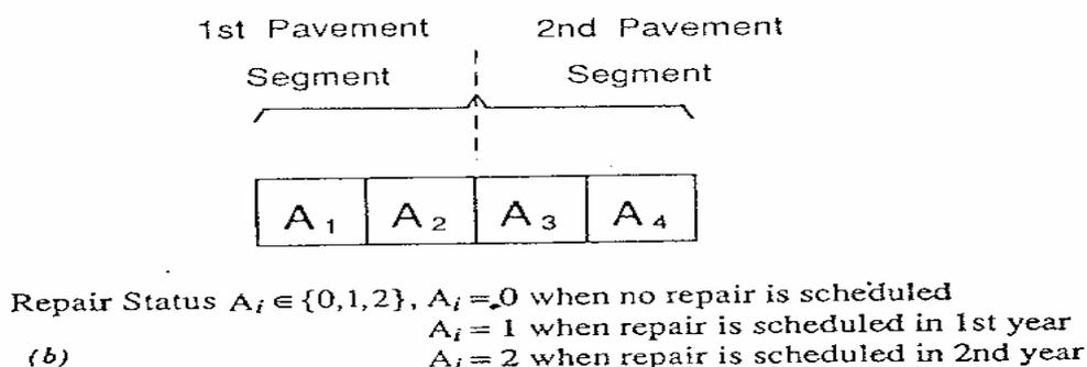
Fwa et al [47] presented the formulation and solution of a genetic algorithms programme, known as PAVENET-R, developed for the programming of pavement maintenance and rehabilitation activities of a road
