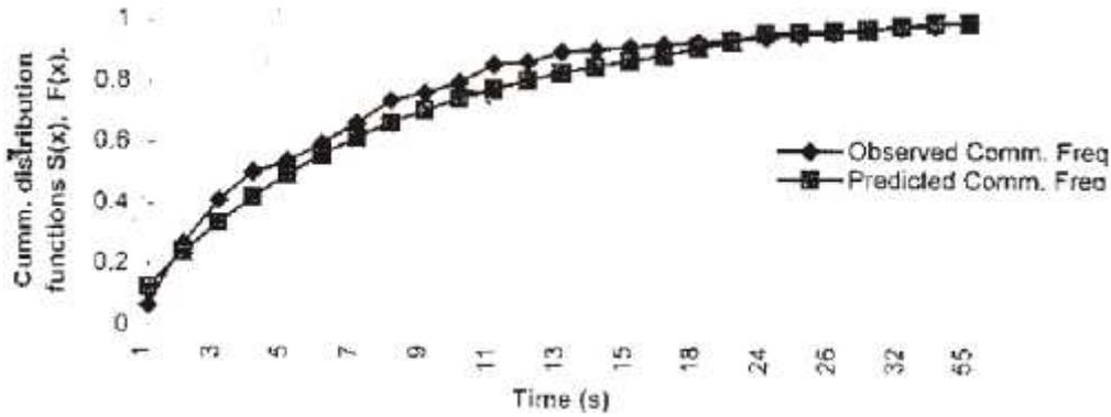
**Figure 3b:** This figure shows observed cumulative frequency versus expected distribution function for bus lanes at 5% level of significance
